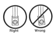
When tightening the screws, be sure to keep bracket parallel to the rail. Otherwise, the rail may bow when opener is operated.
